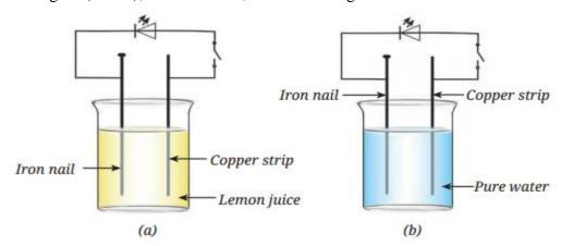
Ans: The LED will glow when the switch is closed in case of (a). Here, the electrolyte is the lemon juice. Copper and iron plates properly placed in a weak acid or salt solution and connected in a circuit produce electricity. In case of (b), the liquid used is pure water that does not become an electrolyte.
