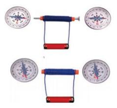
Ans: Yes, the coil will deflect the compass even after the iron nail has been slid out. The coil gets a magnetic force when current flows through it. If an iron nail is inserted inside the coil, the strength of the magnet increases. Deflection in the compass will be less when Neha slides the iron nail out, due to a weaker electromagnet formed by the coil alone.
