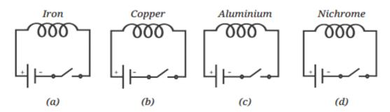
When current is passed through the coils, the compass needles placed near the coils will show deflection.
